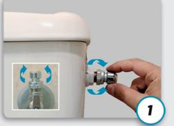
Screw one speed fit in the angle valve that supplies the water and the second speed fit in the basin's water tank.
